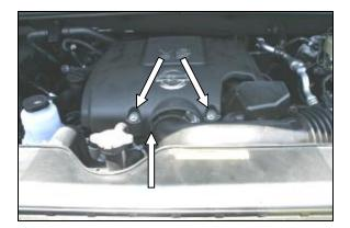
4. Reinstall the factory intake tube, and tighten the hose clamp. Reinstall the engine beauty cover, and tighten the factory bolts. **Re-connect the negative battery cable!**
