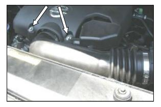
1. **Disconnect the negative battery cable!** Using a 10mm socket, remove the two bolts at the front of the engine beauty cover. Remove the engine beauty cover by lifting up and releasing it from the grommets.
