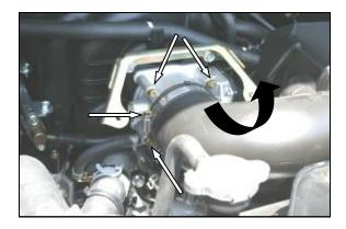
2. Using a 5/16" socket, loosen the hose clamp on the throttle body end of the factory air intake tube. Move the factory air intake tube up and out of the way of the throttle body. Using a 5mm allen wrench, remove the 4 bolts that hold the throttle body to the intake manifold.
